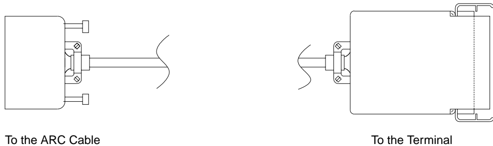
Figure 3-24. French V.35 DTE Adapter
