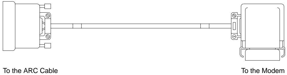
Figure 3-23. French V.35 DCE Adapter
